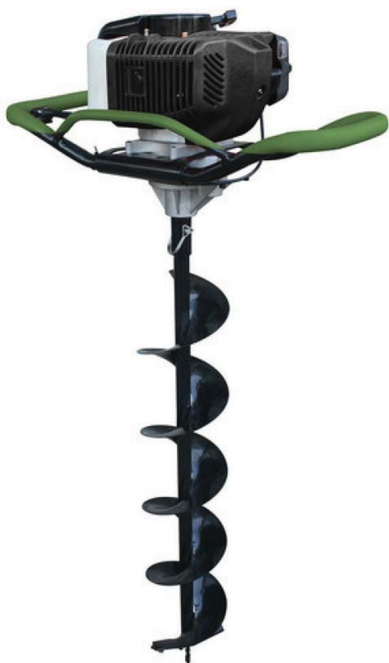
T44G. 6" Earth Series Gas Powered Auger: Easily dig even and consistent holes for fence posts and deck supports with this powerful auger featuring manual recoil start, a 2-cycle engine, 43cc, and 8,500 RPM. 25 points
